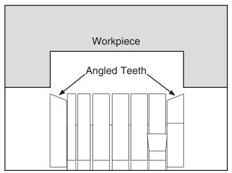
Figure 2. Correct position for outside blades.
